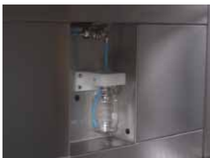
Internal chamber of the pass box with hydrogen peroxide nebuliser
