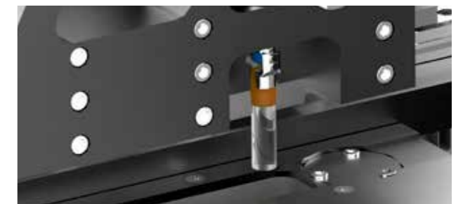
Vial identification, internal code reading
